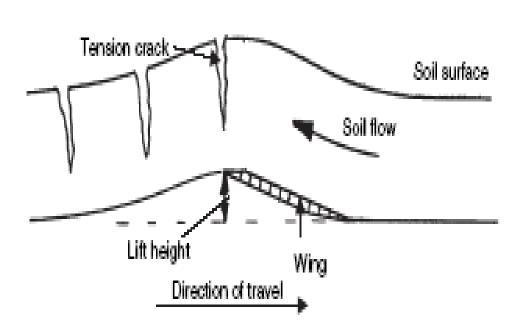
A winged tine of a tiller uplifting a soil to produce tension cracks (Spoor, 2006).
